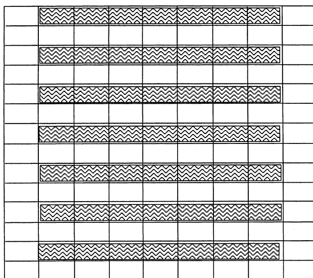
Figure 3 Possible ceiling radiant cooling panel layout in a 1008 ft 2 (94 m 2 ) open office plan example.
